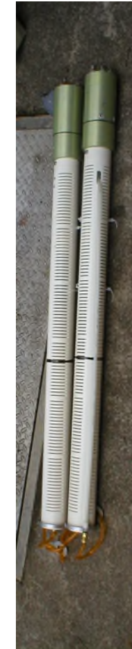
Skimmer pumps and solar powered modular skimmer at DSCP
